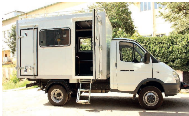
Gazelle brand vehicles maintenance workshop
