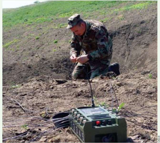
A Moldovan army engineer prepares a radio-controlled system for the remote detonation of explosives.
